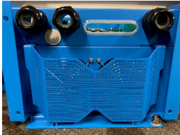
Figure 6 - 5kVA Blue Fan Cover Plate Installed
