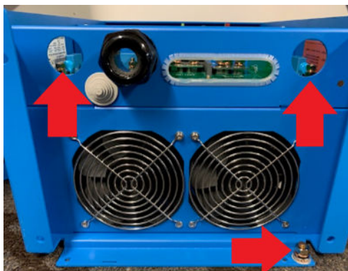
Figure 27 - 5kVA Ground Connection Points
