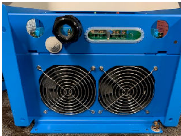
Figure 7 - 5kVA Blue Fan Cover Plate Removed
