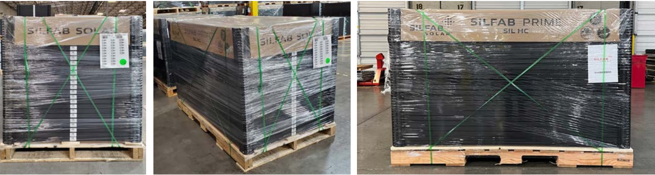
Fig. 7 Horizontal packaging of photovoltaic modules.
